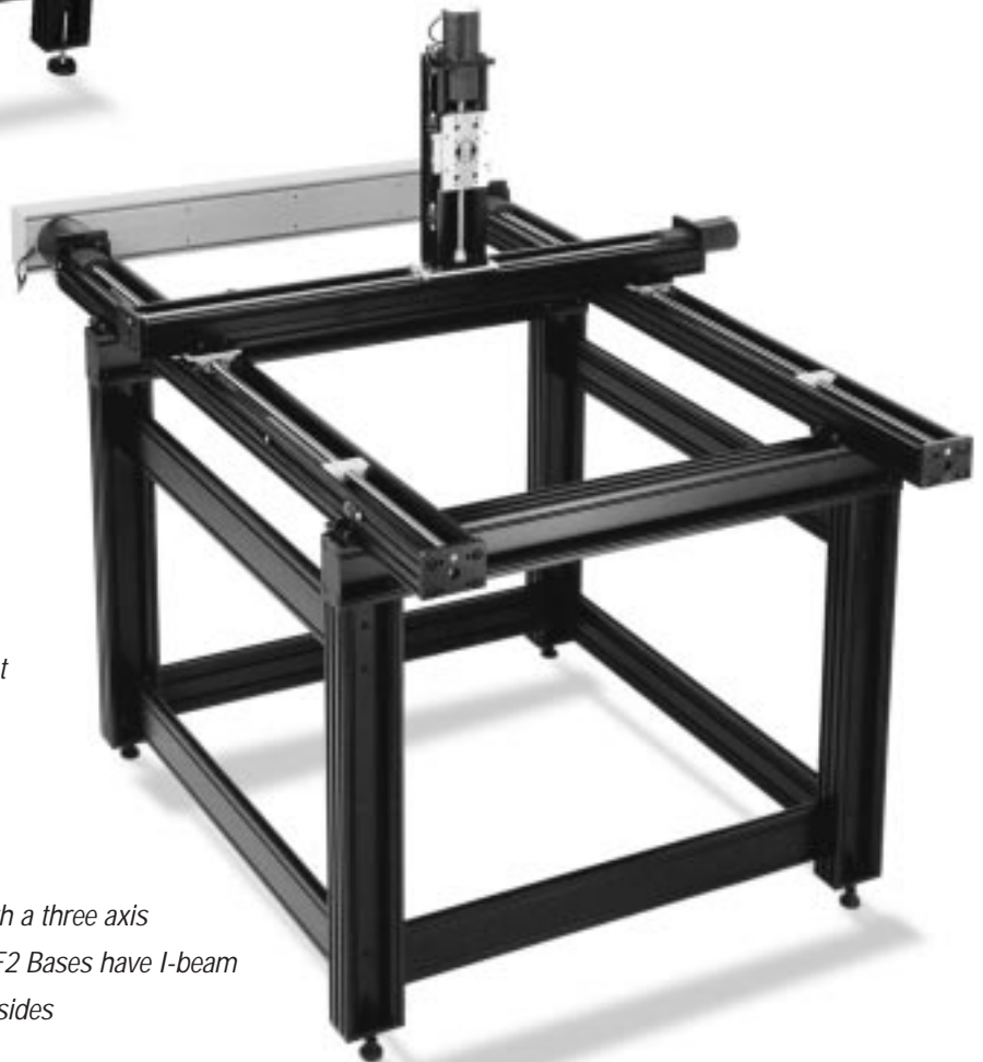
Loads bearing on the top rails are supported directly on the legs, unlike other systems that rely on fastener friction in T-slots for support
