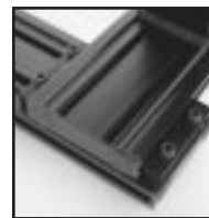
A complete base can be made from T-slot Plate, T-nuts, Bolts, and Cleats
